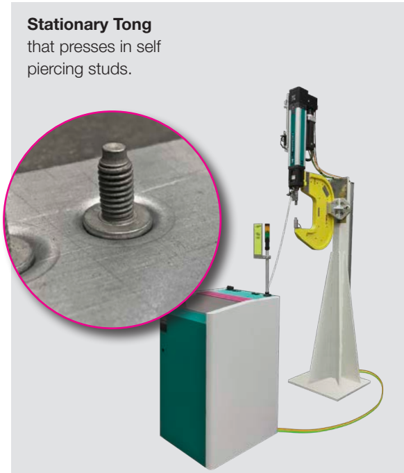
C-Frame Press as a manual workplace. It presses in rivet bolts in a part of a car hood.
