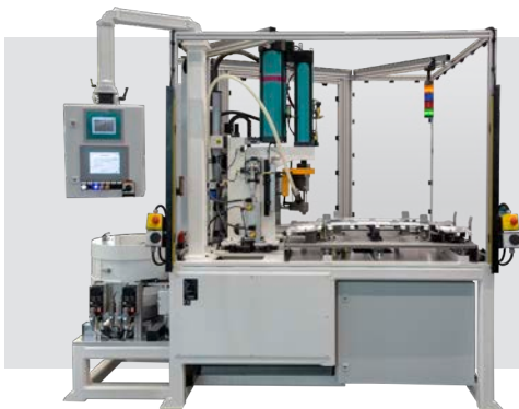
C-Frame Press as a manual workplace. It presses in rivet bolts in a part of a car hood.
